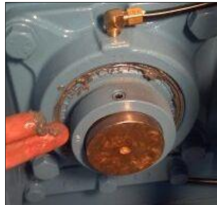
Figure 1. A correctly greased bearing has grease purging around the perimeter.
