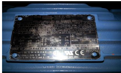
Figure 11. Motor nameplates include wiring legends.
