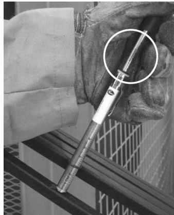
Figure 7. How to measure V-belt tension
