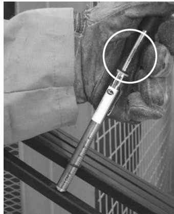
Figure 7. How to measure V-belt tension
