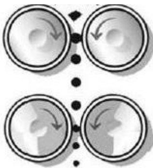
Figure 12. Rolls should spin inwards when motors are spinning counter-clockwise.
