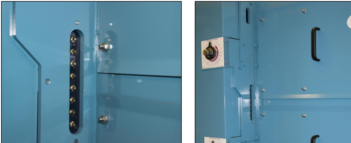
Figure 3. Grease banks located on the front of the machine for easy access
