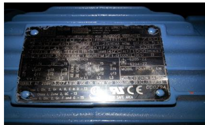
Figure 11. Motor nameplates include wiring legends.
